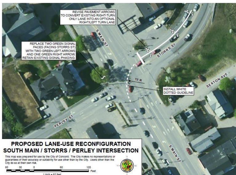
A simple restriping of existing pavement width to add a second left-turn lane at the intersection of South Main and Storrs Streets increased throughput and significantly decreased vehicle delays, resulting in reduced fuel use and air pollution by idling vehicles and reduced driver frustration.
